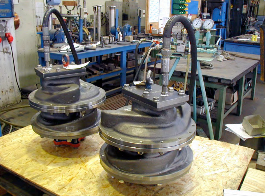
Figure 8: Pressure test of a two stage hydraulic
