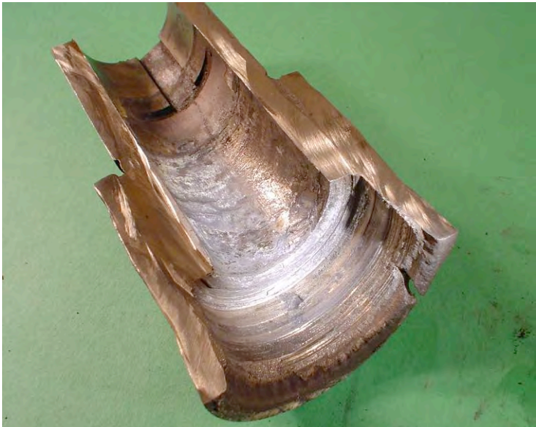
Figure 7: Seized sleeve bearing
