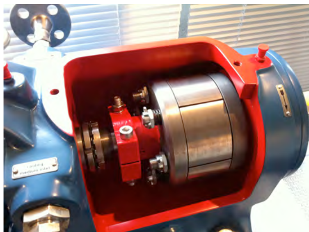
Figure 18: Centrifugal weight assembly with set of springs
