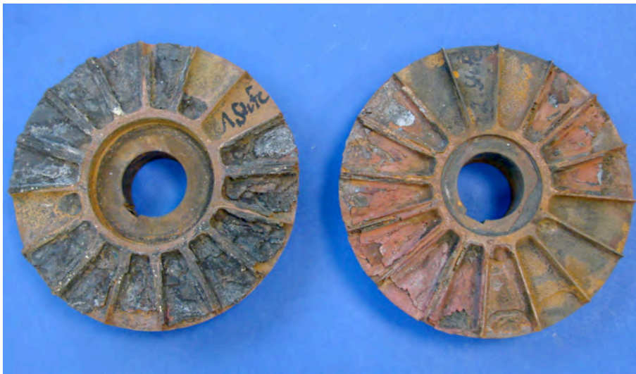
Figure 13: Pyrite deposit on auxiliary impellers
