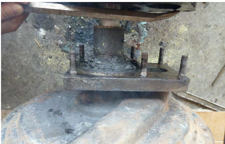
Figure 14: Black pyrite deposit in a foot bearing
